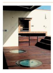
In this duplex **PENTHOUSE** located in Llauder street in Barcelona we installed 2 **DEPLOSUN FLAT-TOP 550** sun pipes leveled with the terrace pavement. Light is transported through the reflective pipe and lightens widely the office-kitchen located in the lower floor and doesn't have any window. The result is a pleasant luminosity feeling and a sensation of connection with the exterior, thanks to daylighting.
